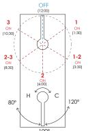
The R1055BD valve has two shared positions. The operation is dedicated and only one outlet will operate at a time.
