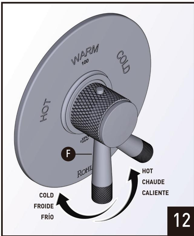
Pull Handle (**F**) and turn clockwise and counter-clockwise to test water temperature.
