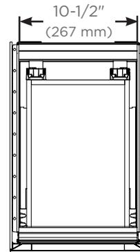
Top view for plumbing and sink clearance
