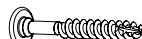
[203-1256] (4) 5/16" x 2 1/2" Structural Bolt (4) 8mm x 63.5mm Boulon (4) 8mm x 63.5mm Perno estructural
