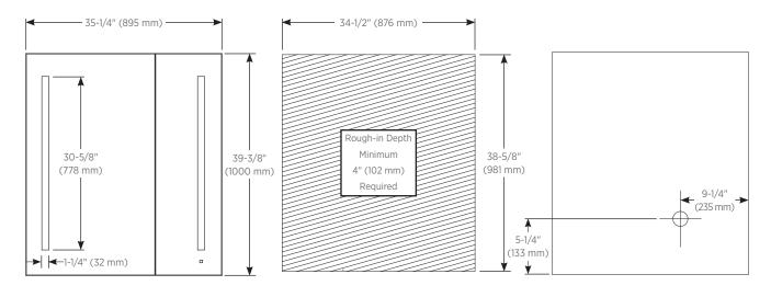
Cabinet Dimensions Rough-in Dimensions Back of Cabinet - Wire Access Location
