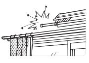
3. Tighten rod cap when in the desired position. 2. Pull out to extend the rod, Rod and push in the rod to contract. Rod support 1. Turn to loosen rod cap.
