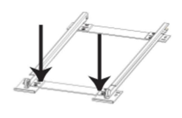
Step 3. Slide drawer out completely and lift drawer out of slide structure.
