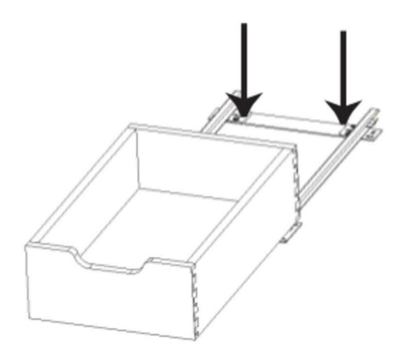
**Step 2.** Slide drawer out half way to allow for installation of rear screws into cabinet floor.
