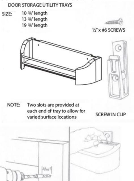
Remove the clips from the tray by disengaging spring hook as shown. Drill pilot holes at locations marked in Steps 1. Wrapping tape 5/16" from tip of a 3/32" drill bit as shown. (Do not drill deeper than front edge of tape). Mount clips at top holes using two (2) 1/2" x #6 screws (do not fasten securely).
