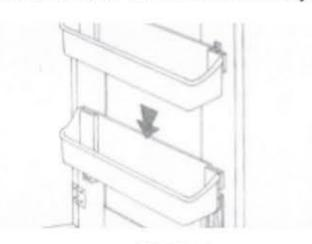
Position the tray on the clips and gently press downward to engage spring lock. This completes the installation of your Door Storage Utility Tray. To install second Door Storage Utility Tray simply repeat Steps 1-4.
