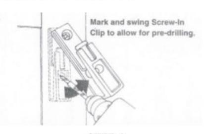
With clips in vertical position, mark bottom hole locations and drill remaining pilot holes (swing clip to allow for drilling). Reposition the clips and securely mount top and bottom of each clip using two (2) ½" x #6 screws. Note: Use plastic screw anchor or #6-32 toggle bolts (available at your local hardware store) when installing Screw-In Clips on wallboard, plaster or very thin material.
