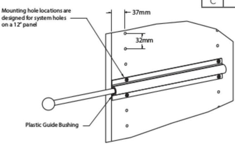
Wood screws can be used if closet does not utilize system holes
