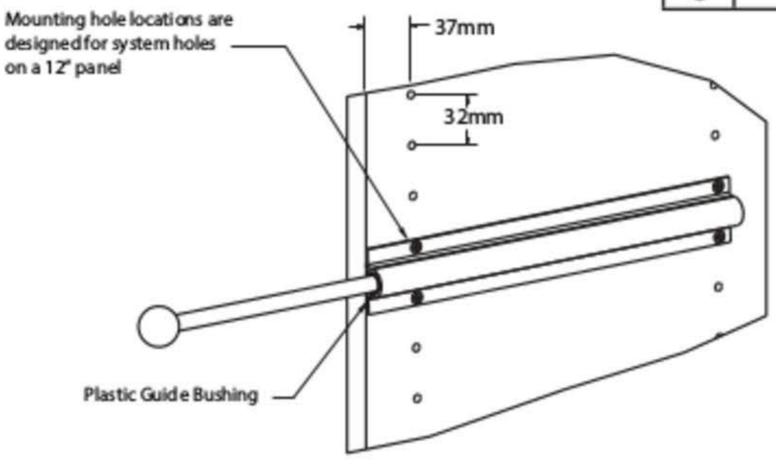
Wood screws can be used if closet does not utilize system holes
