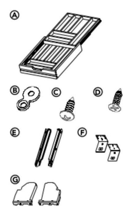
THE MAPLE DRAWER SYSTEM (4WTCD & 4VDO) IS DESIGNED TO USE UNDER MOUNT FULL-EXTENSION DRAWER HARDWARE ONLY. IF YOU ARE REPLACING A DRAWER BOX THAT DOES NOT CURRENTLY USE FULL-EXTENSION (FX) OR PREMIUM GUIDE (PG) HARDWARE YOU WILL NEED TO ORDER A DRAWER GUIDE KIT (DGK).
