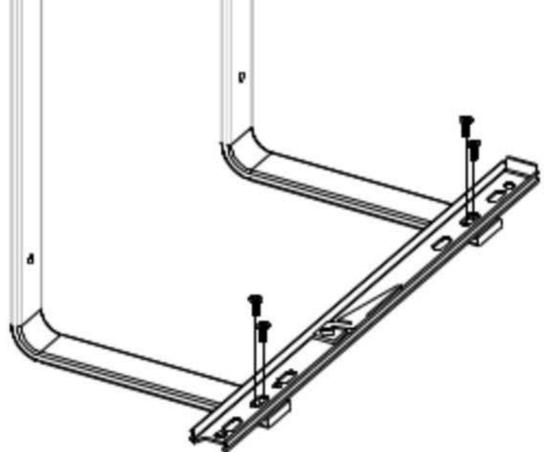
3) Once both inner slides member are attached to both sides you are now ready to attach the brackets to a underside of your shelf using the provided (4) wood screws.
