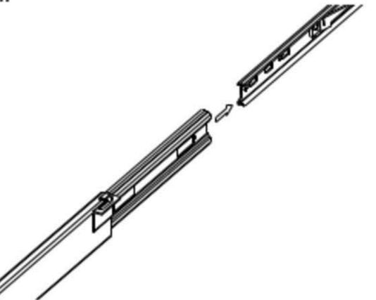
Lay both brackets on one side and attach the inner slide member to the brackets using the provided machine screws.
