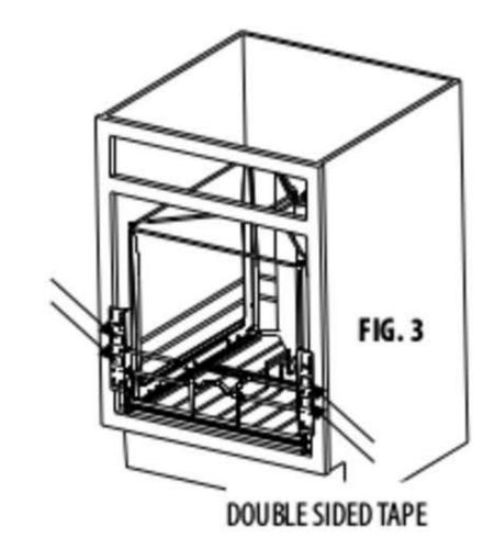
STEP 4) MAKE SURE YOU HAVE CORRECTLY SELECTED THE POSITIONING OF DOOR BRACKET FLANGES SO THAT THE MOUNTING HOLES WILL BE LOCATED IN A PORTION OF THE DOOR THICKER THAN %6".
