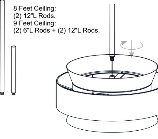
**2 Tighten hex nut inside of the ceiling canopy**
