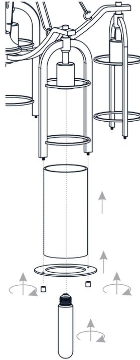
Install five correct bulbs referring to fixture markings and/or labels for maximum wattage.
