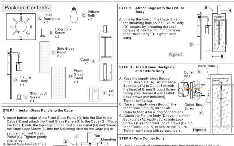
A. Use standard wire connectors (not included) to make all wire connections. (Connectors are not included with fixture.) Twist connectors until wires are tightly joined together. Wrap each connection with approved electrical tape and carefully stuff all the connected wires into the Outlet Box.
