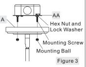
not, adjust the length of the nipple on the Crossbar Assembly (AA) by unscrewing the preassembled hex nut and lock washer and then screwing the mounting screws in or out of the crossbar until the correct length is achieved. Once the Ceiling Canopy (A) is secure, remove the mounting ball and Ceiling Canopy (A) and proceed to
