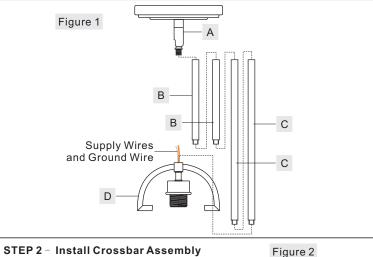
A. Pass the supply wires through the Crossbar Assembly (AA). Attach the Crossbar Assembly (AA) to the Outlet Box with the head of the Green Ground Screw facing you. Secure it with Outlet Box Screws (not included). Tighten until snug.
