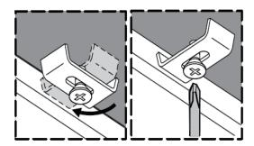
After re-checking alignment, install the clips to the counter top, ensure each clip engages the rim. Tightly and evenly.
