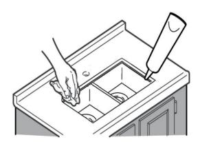
Remove excess sealant and dry for at least 24 hours before use.
