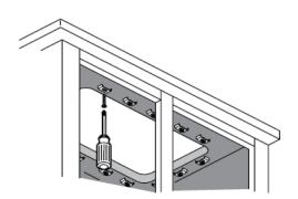
Determine placement of clip brackets as indicated by template. Pre-dill holes according to method desired based on counter top material.
