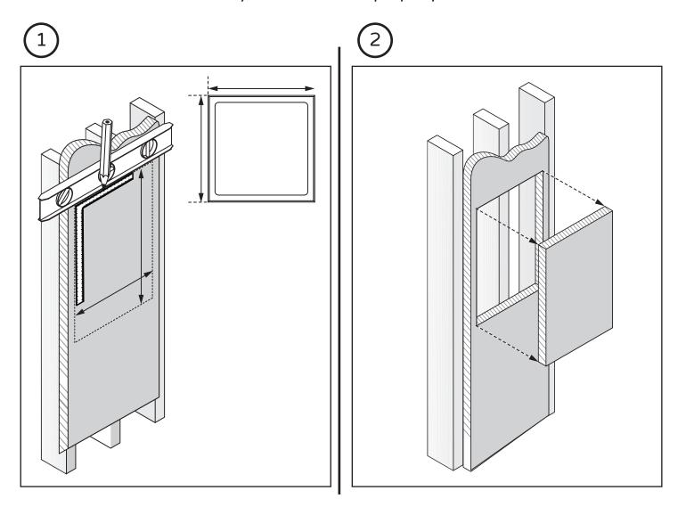
Prepare an opening between the uprights according to the dimensions X and Y of your niche, minus 1/4" (6mm). Ideally, when you insert your niche, it should offer a little resistance in the drywall to prevent it from moving until the silicone dries completely. If you have added another ceramic style finish, make it finish slightly shorter than the drywall.
