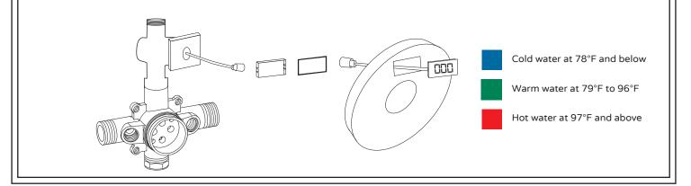
8. Remove plaster guard (19). Install nylon friction ring (17) and wall gasket (21) to trim plate (18). Align trim plate with LED display and slide over valve assembly. Install handle (14) and tighten set screw (15).
