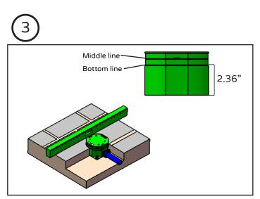
Make sure the mounting base (10) is vertical and centered to you. Tighten mounting base (10) with metal screws (11), make sure floor tile must be higher than bottom line and lower than middle line of mounting base (10).
