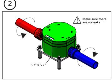
Connect hot and cold water pipes to mouting base (10).
