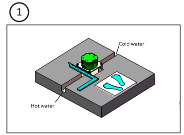
Confirm position for the mounting base (10) and standing place. Suggested distance between them is 30". Dig hole based on the mounting base (10) size.
