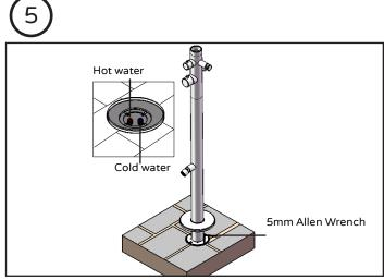
Insert bottom shower pipe (2) to the mounting base (10). Connect bottom flange to mounting base (10) with the four 5mm screws (6), then push down the bottom escutcheon.
