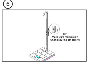
Insert top shower pipe (1) into bottom shower pipe (2). Connect hex head end of hose to swivel joint and tapered end to handshower (4). Place the tapered end of the hose into the handshower holder (9).
