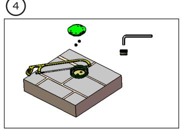
Discard mounting base cover and plugs for hot and cold water outlets. Cut the extra top part of the mounting base (10).
