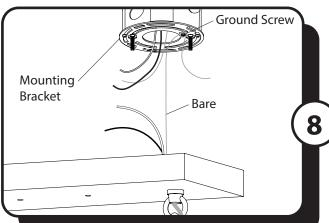
8. Loosen the ground screw on the mounting bracket and wrap the bare wire from the fixture around the ground screw. Tighten the ground screw to hold the bare wire in place. **Note:** Ensure there is enough of the bare wire extending from the ground screw to connect to the ground wire from the outlet box using a wire connector.
