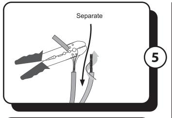
5. Separate the two wires all the way to the canopy. Strip 1/2 in. of insulation from the end of the wires. Twist the stripped ends of each strand of wire within the insulation with pliers (not included).
