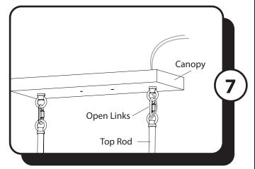
7. Use the two open links to attach the top rods to the chain loop. Feed the wires from the top rod through the canopy.
