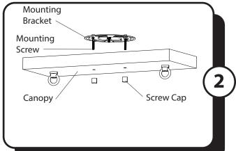
2. Remove the screw caps from the mounting screws preassembled to the mounting bracket. Remove the mounting bracket from the canopy.
