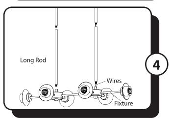
4. Determine which combination of short rods and long rods to use, based on the desired length of the fixture. Install top rods with loops last as they will be used to hang the fixture on open links. Twist the wire ends coming from the fixture together and feed through hole in the first rod. Connect the first rod to the fixture by twisting the threaded end onto the fixture in a clockwise direction until secure.
