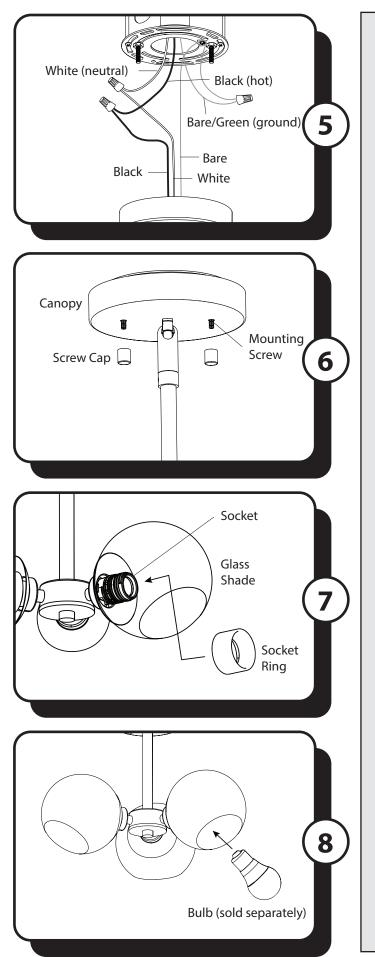
5. Use wire connectors to secure the household supply wires to the fixture wires according to the image and the following instructions:
