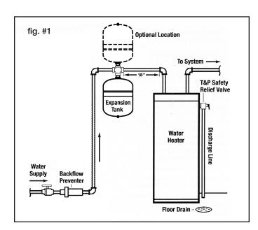
Before turning on the water supply to the system, open a hot water faucet to prevent any damage to the water heater and remove air from the system piping. Turn on the water supply and inspect the installation for water leaks paying close attention to the connection between the expansion tank and the piping.
