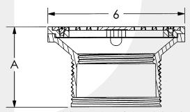
• Barrel diameter is 3-1/2 in. IPS thread.
