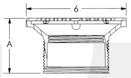
• Barrel diameter is 3-1/2 in. IPS thread.
