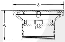
• Barrel diameter is 3-1/2 in. IPS thread.
