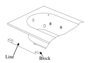
7. For final skirt installation and to allow for removal if necessary in the future, adhere skirt to wooden back support blocks with silicone or other removable adhesive. Place a straight board against front bottom of skirt to hold it firmly in place while the adhesive cures.
