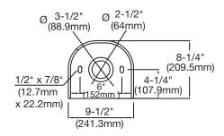
Note: All dimensions and specifications are nominal and may vary: Dimensions of 8" and greater have a tolerance of +3%. Dimensions less than 8" have a tolerance of +5%.
