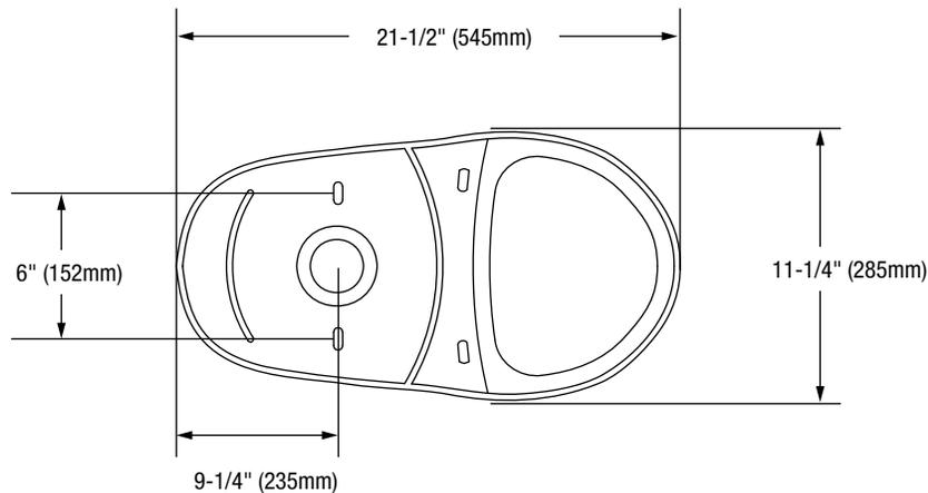
Note: All dimensions and specifications are nominal and may vary: Dimensions of 8" and greater have a tolerance of +3%. Dimensions less than 8" have a tolerance of +5%.
