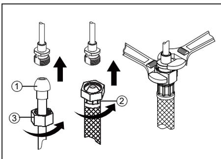
2. Make connections to water lines. Use 1/2" I.P.S. faucet connections (2) or use supply line coupling nuts (3) with 3/8" O.D. ball-nose riser (1). Use wrenches to tighten connections. Do not over tighten.
