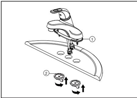
1. Shut off main water supply before installation. Remove old faucet. Place gasket (1) on bottom of new faucet. Place faucet through mounting holes in sink. Secure faucet to sink using mounting nuts (2) provided. Remove the sleeve from the inlet tube.
