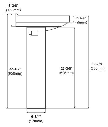
Note: All dimensions and specifications are nominal and may vary: Dimensions of 8" and greater have a tolerance of +3%. Dimensions less than 8" have a tolerance of +5%. Please utilize the current cutout template for countertop cutouts.
