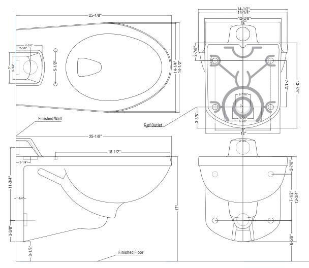
All dimensions and specifications are nominal and may vary. Dimensions of 8" and greater have a tolerances of +3%. Dimensions less than 8" have a tolerances of +5%.
