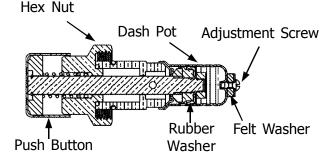
**To Install:** Remove old flush valve assembly and make sure the valve is free from debris or defects. Install flush valve into the assembly and tighten. Tighten to 90 in/lbs pressure.
