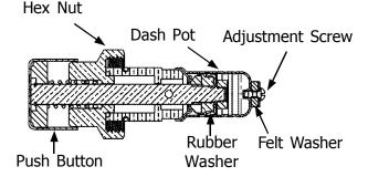
**To Install:** Remove old flush valve assembly and make sure the valve is free from debris or defects. Install flush valve into the assembly and tighten. Tighten to 90 in/lbs pressure.
