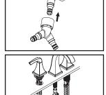
(4) Place cold and hot side valves in position on the sink, ensure handles operate in correct direction. From underneath the sink, hand-tighten locknut to the side valve. Position side valve to desired location from top. Tighten screws on locknut with the help of Phillips head screwdriver to secure side valve.
