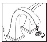
(6) Important: After installation is complete, remove the aerator. Turn on the water and allow both hot and cold water to run for at least one minute each. While water is running, check for leaks. Turn off the water and replace the aerator when finished.
