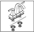
(2) Place the faucet in position on the sink. Install washer on shanks and tighten with locknut.
