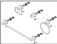
(3) Secure the bathroom hardware with the screw at the bottom. Do not overtighten.
