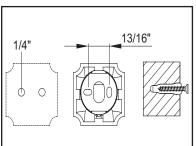
(1) Determine the installation location for the bathroom hardware. Drill 1/4" diameter hole approximate 13/16" apart. Place plastic anchors into the drilled holes, use hammer to tap it in flush with the wall. Place the mounting plate and secure them to the wall with the help of mounting screws.
