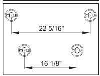
(2) For 7PR030 & 7PR031 Install the mounting plate 22-5/16" & 16-1/8" apart respectively.
