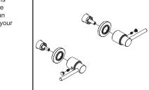
(6) Slide valve escutcheon through valve sleeve, attach hot and cold handles to the cartridge and tighten with Allen screw, put hole cover on both handles.
