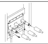
(4) Connect water supply lines to faucet inlet tube. If using copper pipe, please remove both hot and cold side stems before soldering the pipes. Reinstall both hot and cold side stems after soldering the pipes. Turn on both stems to flush the system and check for any leaks. Please put the protection tube on the rough-in valve if the finished wall is not done yet.
