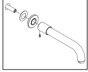
(5) When the finished wall is done. With spout escutcheon and gasket in the back, push spout and escutcheon through spout shank against the finished wall then tighten the Allen screw on the spout. Use silicon to caulk around valve escutcheon and spout escutcheon to form water tight seal.
