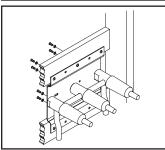
(3) Attach the wall bracket to the framing with six mounting screws provided with the wall bracket. Verify that the installation is correct and leveled. Also verify the wall bracket is firmly secured to the framing
