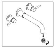
(7) Important: After installation is complete, remove the aerator. Turn on the water and allow both hot and cold water to run for at least one minute each. While water is running, check for leaks. Turn off the water and replace the aerator when finished.
