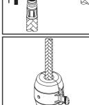
(6) Install weight on spray head hose. Adjust weight's position so the spray head can be retracted properly.
