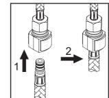
(5) Insert spray head hose into end of quick connect adapter on the outlet hose, push until a "click" is heard. Pull down to test
