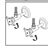
(7) Connect hot and cold inlet supply hoses to supply stops. For supply stop with 1/2" outlet connection, use 3/8" male to 1/2" female adapter for installation. Adapters are optional and are not provided with the faucet. Turn on both side supply stops to check any leaks.
