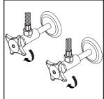
1) Shut off the water supply. Remove old faucet. Clean mounting surface in preparation
