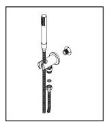
(1) Apply Teflon tape to the pipe nipple stretching out from the wall, attach drop ell with handheld support to pipe nipple. Install vacuum breaker to drop ell. Connect 60" stainless steel hose to vacuum breaker. Use silicone sealant to caulk around drop ell to create water tight seal. Turn on water and check for any leaks. Turn off water and connect handheld showerhead to 60' stainless steel hose.
