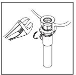
(3) Insert pop-up flange through drain hole and attach flange to the pop-up drain body. Apply Teflon tape on the threaded end of the tail piece and attach tail piece to the pop-up drain body. Ensure the pivot rod hole of the pop-up drain body faces towards the back of the sink. Tighten the locknut with the help of a wrench to secure the pop-up drain body.
