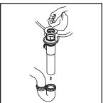
(4) Remove the excess plumbers putty. Connect the trap (check manufacturer's instructions for installation).
