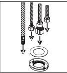
(4) With flat side of the locknut facing down and the steel washer inside the locknut please follow the order as the drawing shows to insert flex hoses through the center hole of the locknut from underneath the sink.
