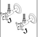
(8) Connect hot and cold inlet supply hoses to supply stops. For supply stop with 1/2" outlet connection, use 3/8" male to 1/2" female adapter for installation. Adapters are optional and are not provided with the faucet. Turn on both side supply stops to check any leaks.
