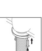
(5) Thread locknut onto the faucet shank from underneath the sink. Position faucet to desired location from the top and hand-tighten locknut till it won't go further. Thread both screws on locknut and tighten screws on locknut with the help of a Phillips head screwdriver to secure faucet. (Note: Do not overtighten.)
