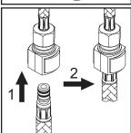
(7) Insert spray head hose into end of quick connect adapter on the outlet hose, push until a "click" is heard. Pull down to test engagement.
