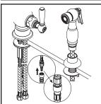
(4) Guide the side spray hose through the side spray holder. Insert the side spray hose quick connect adapter into the faucet outlet hose end, push until a "click" is heard. Pull side spray hose downward to test engagement.
