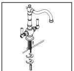
(2) Thread and tighten mounting bolt to the bottom of faucet, place escutcheon with washer under the faucet, insert faucet through mounting hole. Slide mounting washers to the mounting bolt and tighten mounting nut to mounting bolt from underneath the sink. Go to step (5) if faucet is without side spray.
