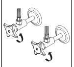
(5) Connect hot and cold inlet supply hoses to supply stops. For 1/2" connection; use 3/8" male to 1/2" female adapter for installation. Adapters are optional and not provided with the faucet. Turn on both sides of the supply stop.
