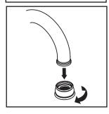
(5) Important: After installation is complete, remove the aerator. Turn on the water and allow both hot and cold water to run for at least one minute each. While water is running, check for leaks. Turn off the water and replace the aerator when finished.
