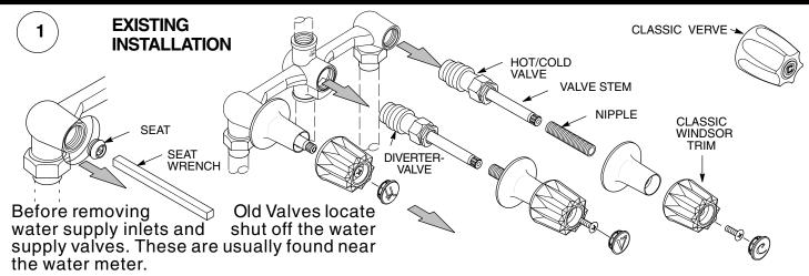
For removal of Hot and Cold water valves be sure Stems are in full ON position and water is turned **off**. Remove trim, flanges, nipples, valves, and seats.
