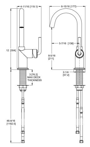
36 Inch Supply Lines with 3/8 Female Compression Brass Connections
