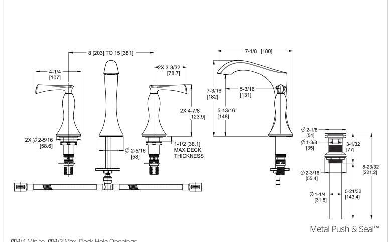
Ø1-1/4 Min to Ø1-1/2 Max. Deck Hole Openings
