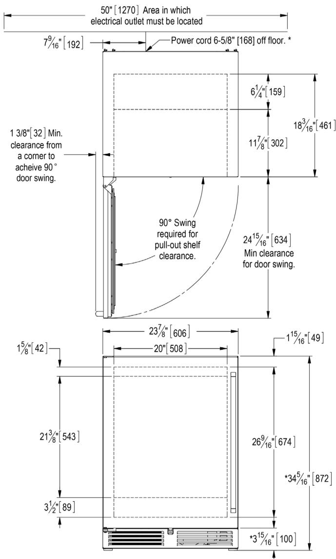
\* - Leg levelers can add 3/4" [19] to these dimensions when fully extended.
