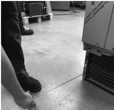
Adjusting front leveling legs.
