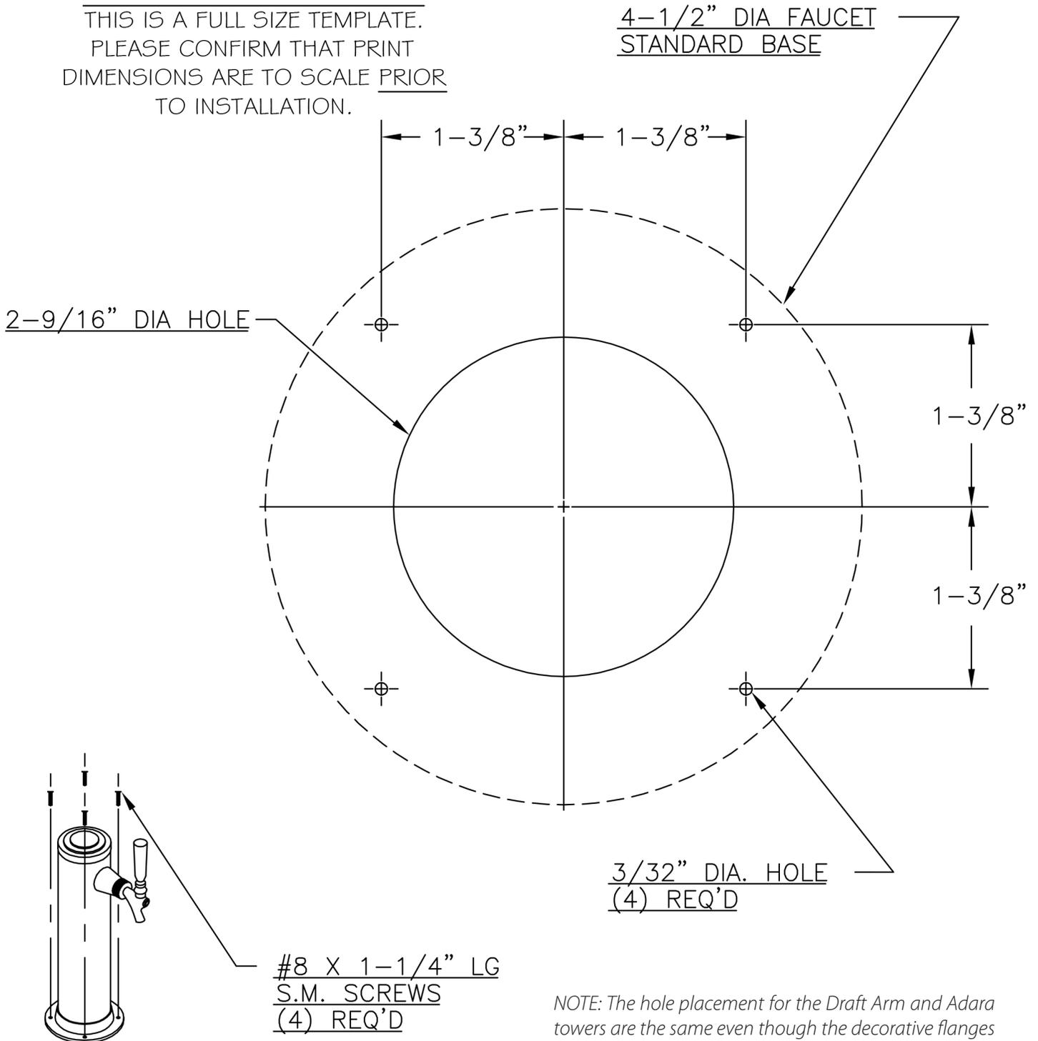
*NOTE: The hole placement for the Draft Arm and Adara towers are the same even though the decorative flanges are different shapes.*
