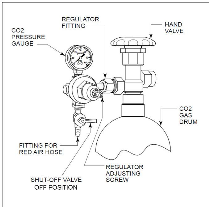
1. Remove the blue plug from the regulator fitting, but do not remove the carbonic washer.
