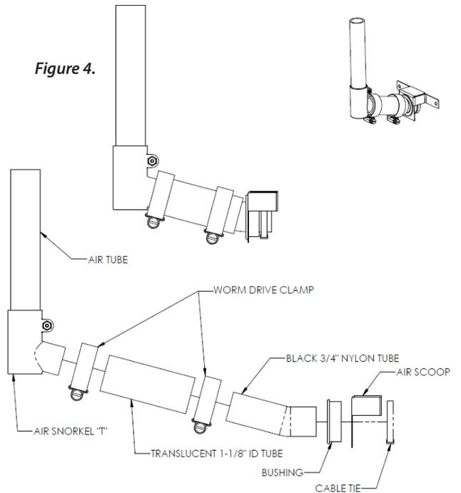
2. Remove air "T" from end of air tube by loosening fastener holding the two halves together. Remove the air tube from the tower being careful not to damage the product tube.
