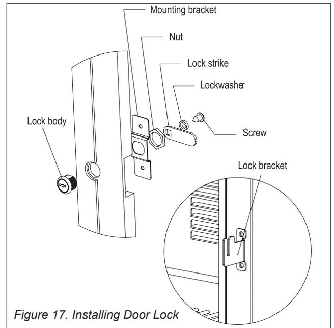
Figure 17. Installing Door Lock
