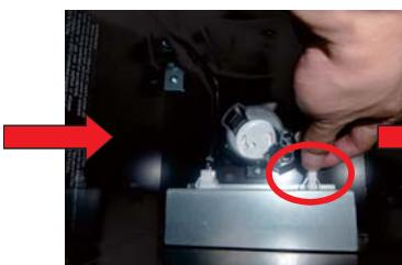
Unplug light unit assembly connector, Then take out the whole assembly
