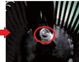
Remove the blade fixing nut
