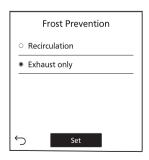
Frost prevention operations "Recirculation" and "Exhaust" are compatible with FV-16VEC1/T and FV-13VEC1T/S models.
