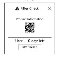
3 Press the button to reset the countdown for the next maintenance.
