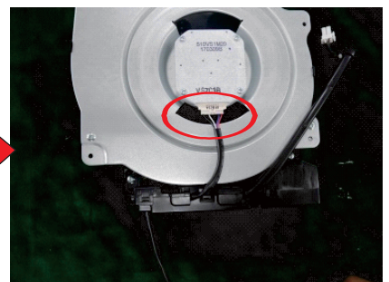
Pull out the motor lead from motor assy
