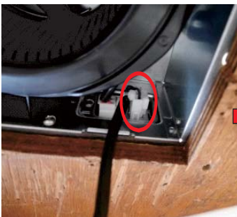
Unplug led unit connector , Then take out the louver assy
