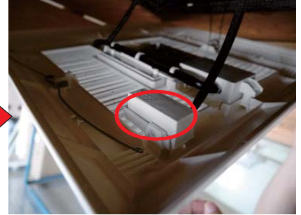
Remove the humidity sensor assy
