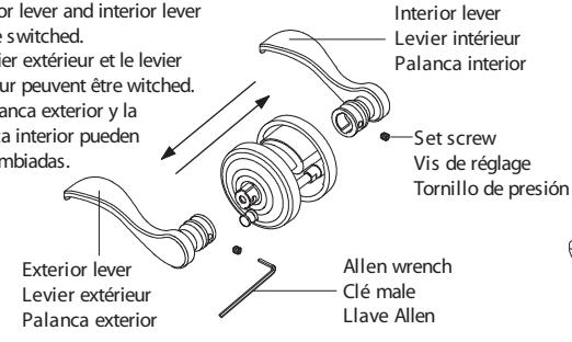
Using Allen wrench to firmly tighten set screws.
