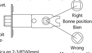
B. To convert latch to 2-3/4"(70mm) backset, pull the rear part until 2-3/4"(70mm) is completely shown in indicator.
